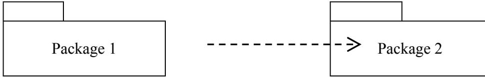
**Figure 13: UML notation for two collapsed packages with a dependency relationship**
