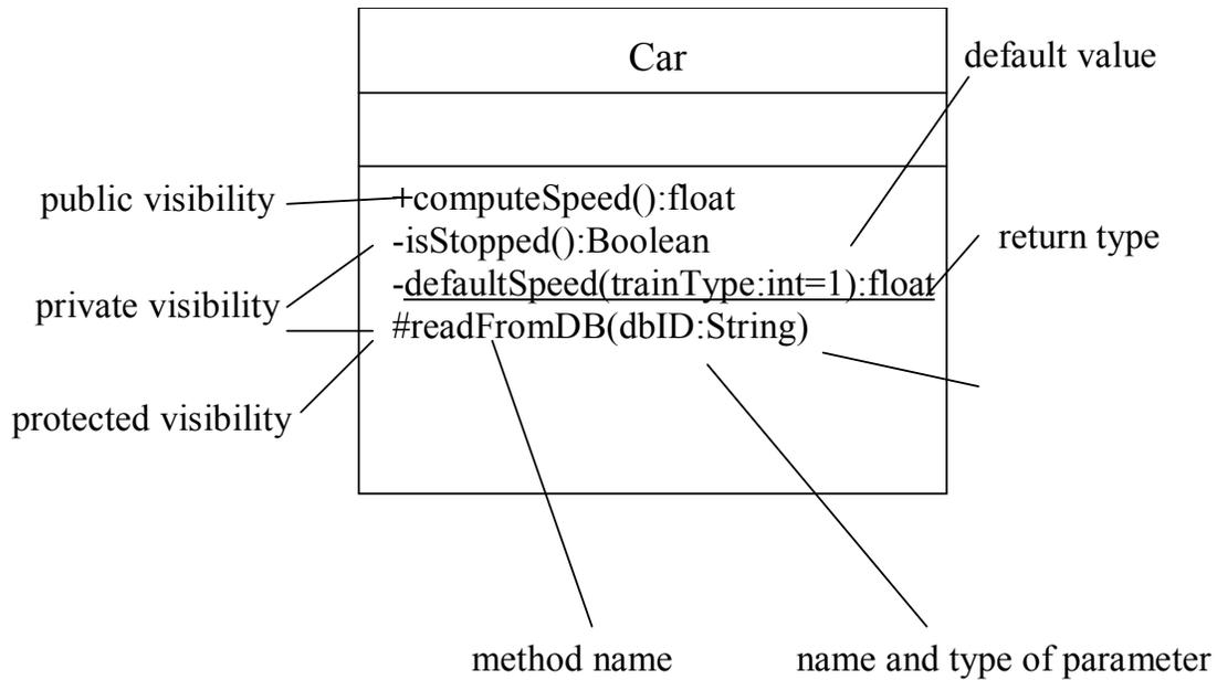
Figure 11: UML notation for operations/methods
